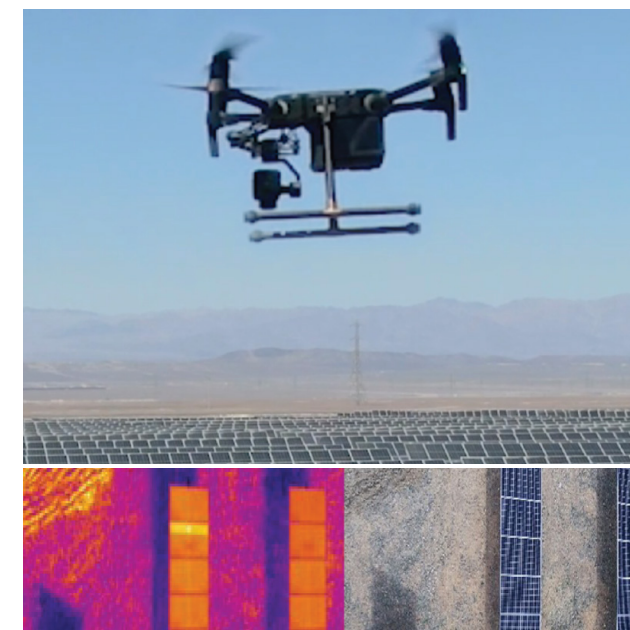
Figure [1] : Drone flying over solar farm and infrared inspection shots taken by on-board came
